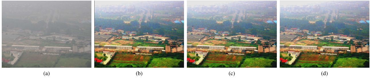
Fig. 6: Results of fog removal algorithm of optimization and vectorization. (a) Original 'test1' Image, result of (b) OFR algorithm, (c) FRPO approach, (d) FRPOV approach.
