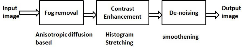
Fig. 1: Block diagram of fog removal algorithm
