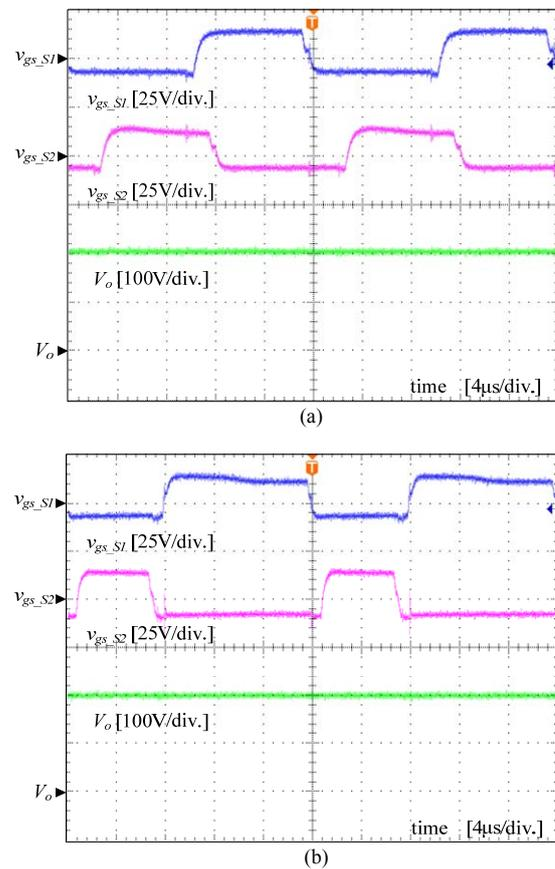
Fig. 7. Experimental waveforms for the gate signals and output voltage according to the operation mode. (a) PSFB series-resonant converter mode when  $V_d=350$ V. (b) Active-clamp step-up converter when  $V_d=250$ V.
