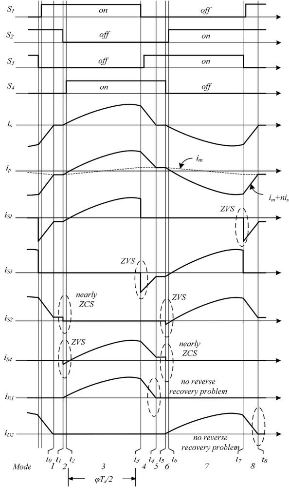
Fig. 2. Operation waveforms in the PSFB series-resonant converter mode.
