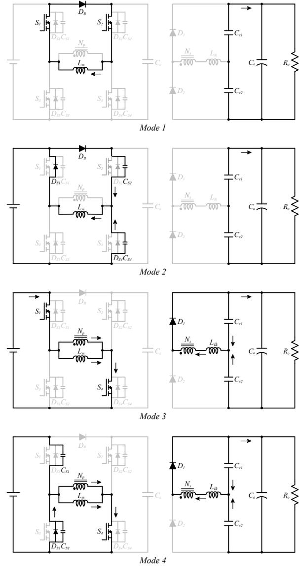
Fig. 3. Equivalent circuits during half period in the PSFB series-resonant converter mode.
