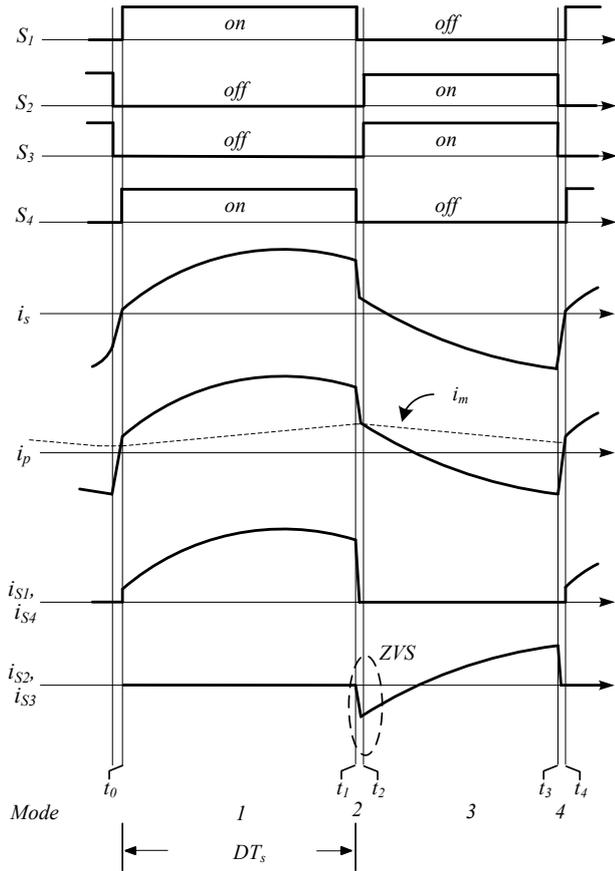
Fig. 4. Operation waveforms in the active-clamp step-up converter mode.
