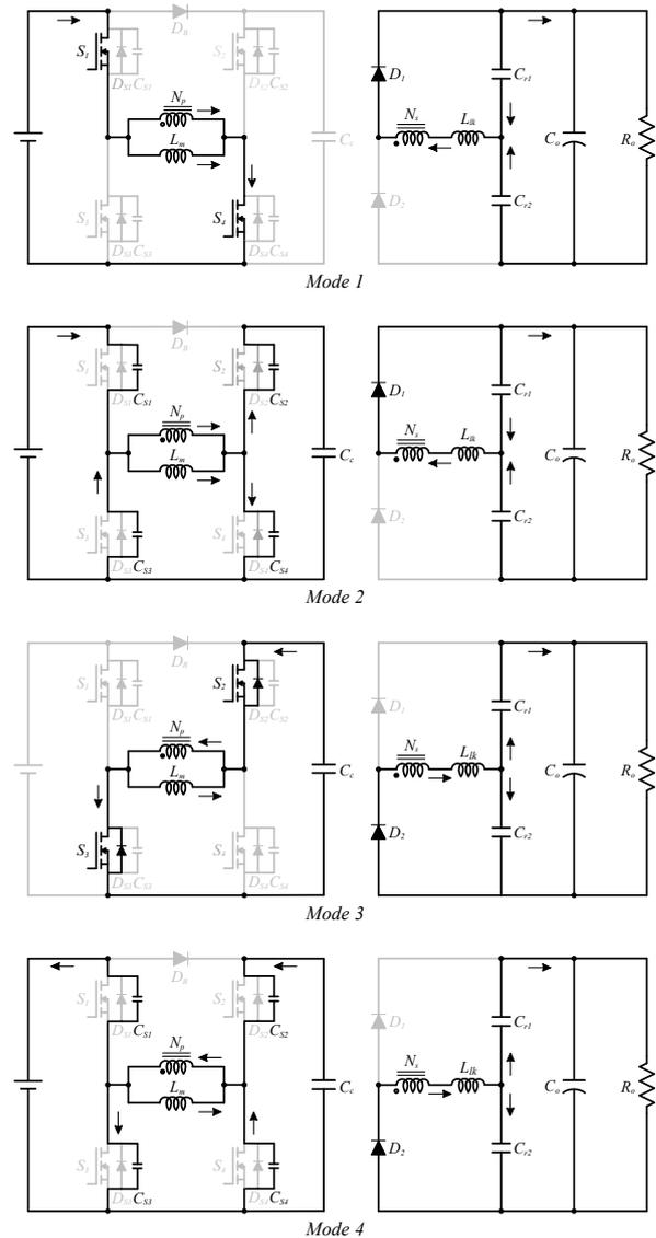
Fig. 5. Equivalent circuits during a switching period in the active-clamp step-up converter mode.
