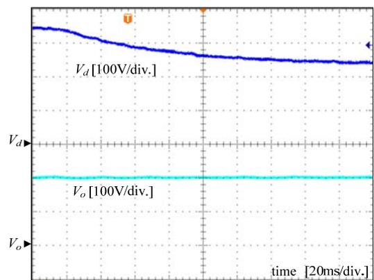
Fig. 10. Experimental waveforms for the input voltage  $V_d$  and output voltage  $V_o$  in the transition-state.
