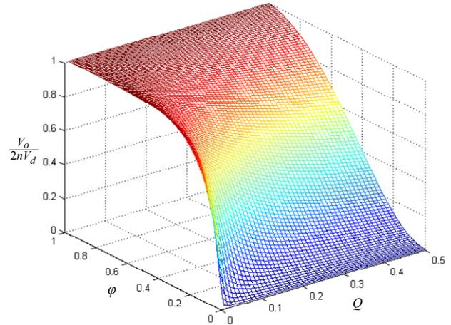
Fig. 6. Normalized voltage gain at  $F=1.05$  in the PSFB series-resonant converter mode.
