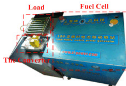
Fig. 11. Prototype of the 1 kW Converter with Fuel Cell and Load
