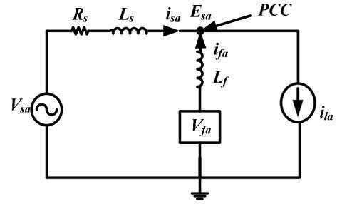
Figure 2. Single-phase equivalent circuit of APF topology
