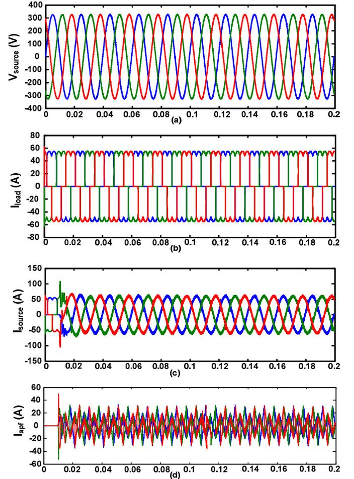
Figure 6. Simulation results (a) Source voltages, (b) Load currents, (c) Compensated source currents, and (d) Filter currents (APF).
