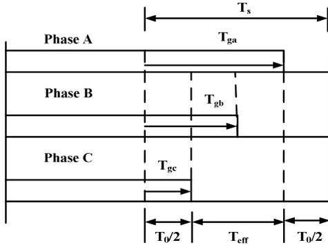
Figure 5. Proposed shunt APF switching pattern
