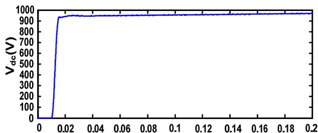
Figure 7. DC Bus voltage of the proposed shunt APF
