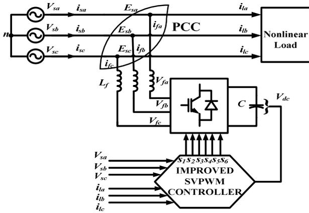
Figure 1. Configuration of Improved SVPWM based shunt APF
