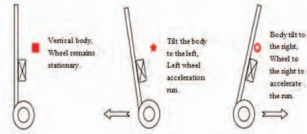
Fig 3. Platform balance control process. Controlling wheel rotation and offsetting incline trend in one dimension can keep body balance.
