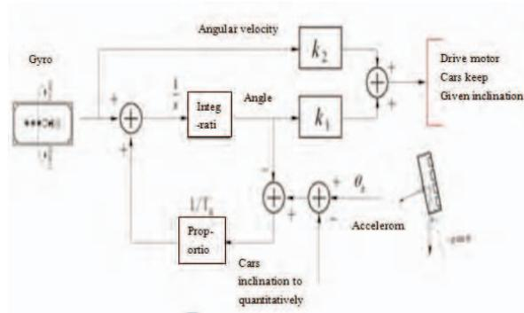
Fig 5. Control flow. Given platform upright control set point, the platform will automatically maintained at an angle under the angle control adjusting.
