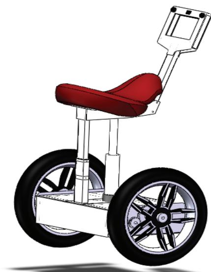
Fig 6. Platform walking. Mobile platform is flexible and convenient, it can enter the elevator and run on the small slope.
