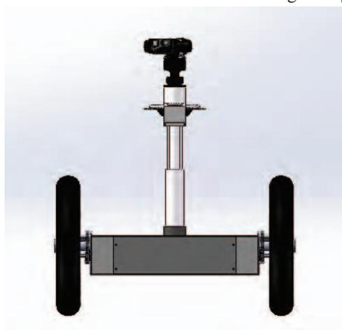
Fig 7. Platform carrying photographic equipment. Platform can carry three degrees of freedom adjustable pan-tilt.
