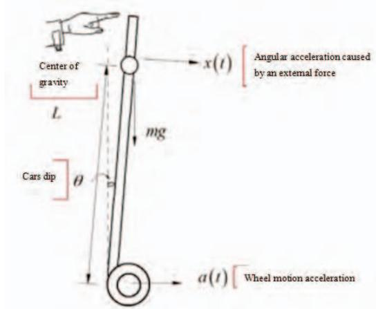
Fig 4. Platform can be simplified into a pendulum, whose height is L, mass is m.
