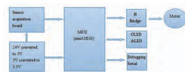
Fig 2. Hardware circuit diagram of the system. The system is mainly composed of main control chip and sensors.
