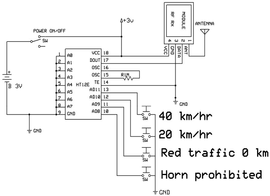
Fig. 1. Transmitter Circuit
