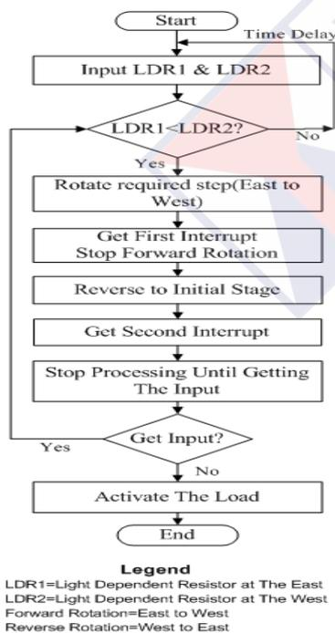
Fig. 3 System implementation flowchart of the single axis tracker
