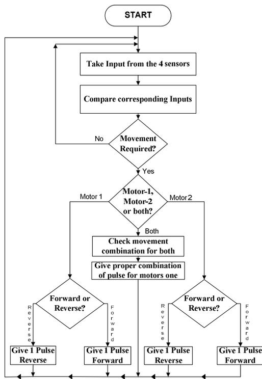
Fig. 5 System implementation flowchart of the dual axis tracker [4]
