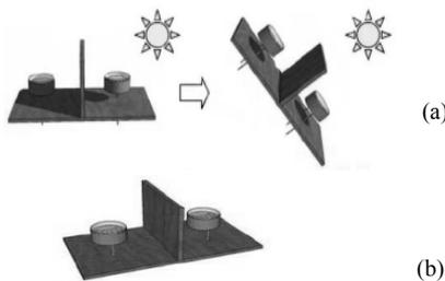
Fig. 2 (a) Sensor module; (b) Operation of sensor module once an LDR comes under shadow [8]
