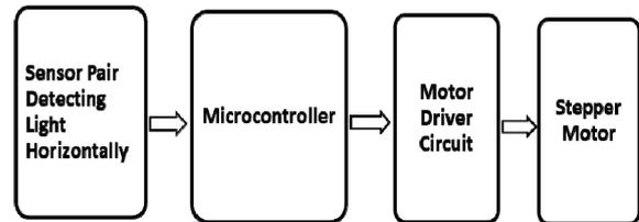
Fig. 4 Block diagram of automatic single axis solar tracking scheme
