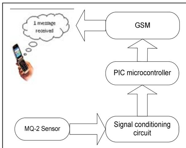
Fig. 1 Block diagram of haze monitoring process
