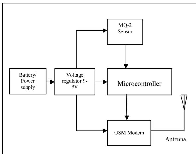
Fig. 2 Block diagram of transmitter
