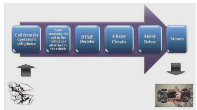
Figure 1. Block diagram of GSM network controlled vehicle.
