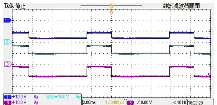
(c) Waveform of RGB duty cycle (R=30%, G=30%, B=30%)
