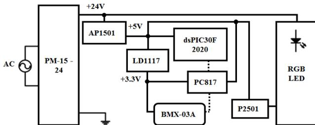
Fig. 5 Block diagram of the proposed system
