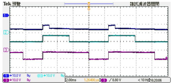
(a) Waveform of RGB duty cycle (R=10%, G=40%, B=70%)
