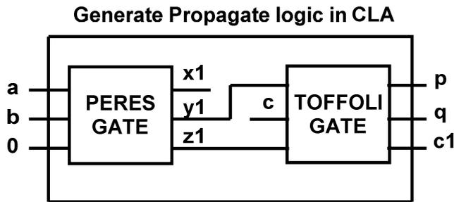
Figure.10 Generate propagate logic in CLA
