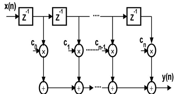
Figure.1 Direct form FIR Filter structure
