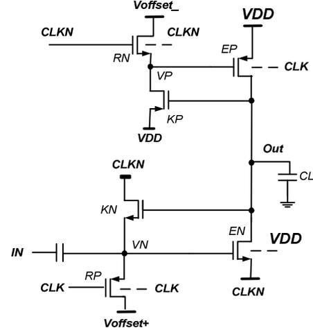
Fig 3. the Bulk of the Precharge devices are stimulated with the clock and the bulk of EN is connected to VDD.
