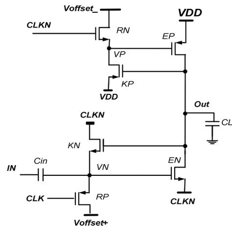
Fig. 1 Simple FGULV Domino inverter. (Precharge to 1).
