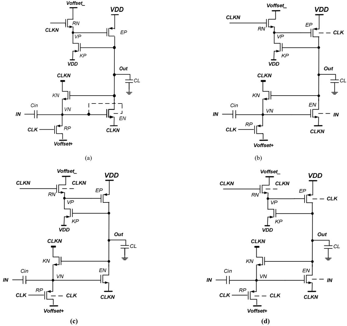
Fig. 2. Different domino FGULV inverters with bulk stimulating technique (a) Bulk of EN is connected to floating gate node (VN) (b) Bulk of EN is connected to the Input and the bulk of the EP devices is connected to the CLK signal. (c) Bulk of the RN is connected to the CLKN and the bulk of the RP is connected to CLK (d) The bulk of the precharge and evaluate devices are manipulated.
