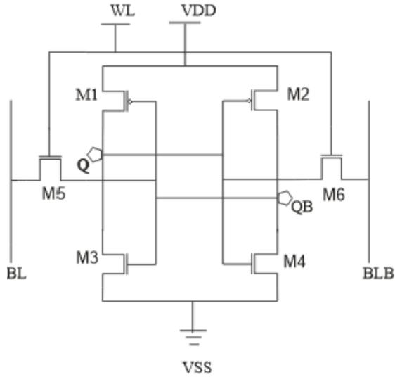
Fig.2 Architecture of Standard 6T SRAM cell.
