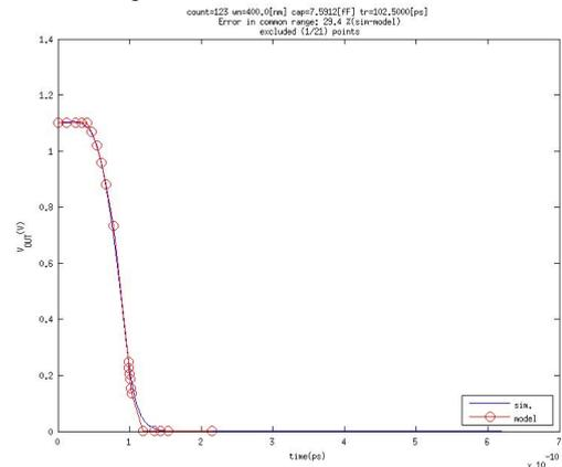
Fig. 4 Output voltage comparison for a NAND gate and for a rising input
