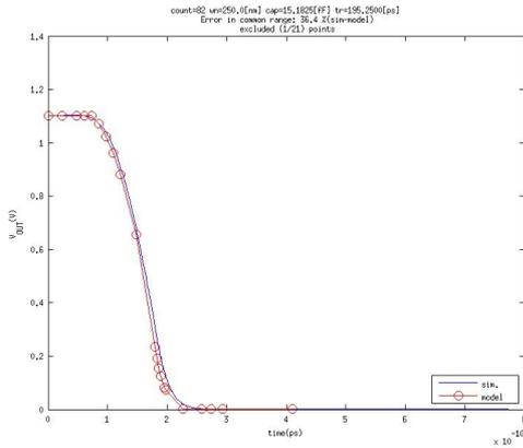
Fig. 2 Output voltage comparison for a CMOS inverter and for rising input
