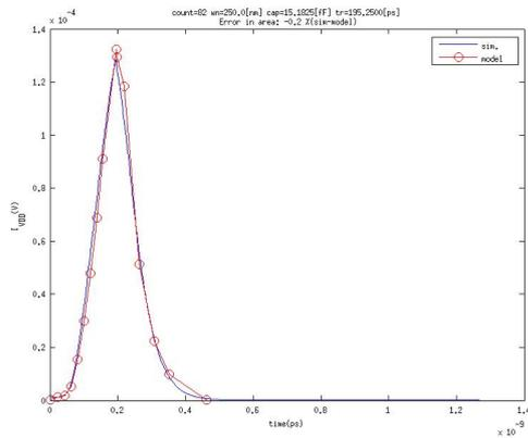
Fig. 3 Supply current comparison for a CMOS inverter and for falling input
