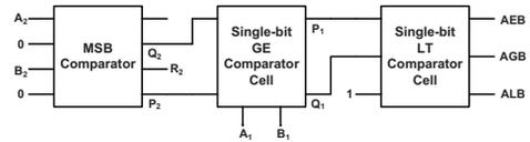
Fig. 7. Proposed Reversible 2-bit comparator
