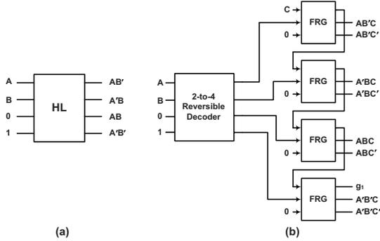
Fig. 5. Proposed Reversible (a) 2-to-4 Decoder (b) 3-to-8 Decoder
