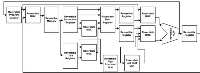
Fig. 2. Datapath Design of the Proposed Reversible Processor
