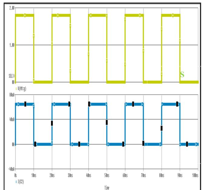
Fig. 5. Output current level for pass transistor architecture of 1:2 de-multiplexer 1.8V VDD
