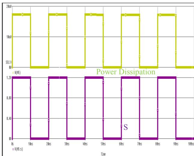
Fig. 8. Characteristic curve of power dissipation for pass transistor architecture of de-multiplexer 1:2 at 1.2V VDD.
