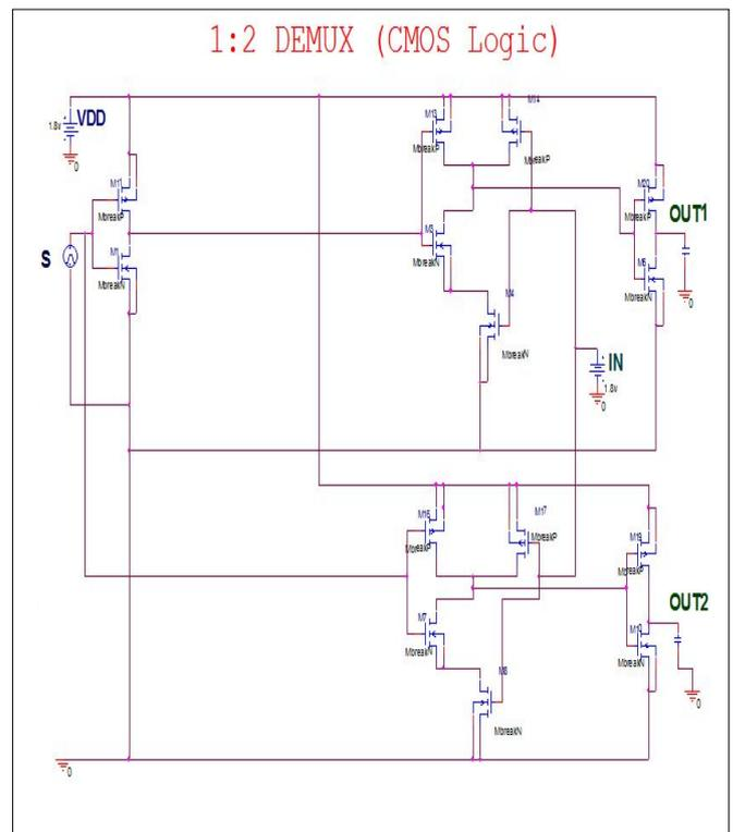
Fig.2. Schematic diagram of CMOS logic configuration of 1:2-demultiplexer.
