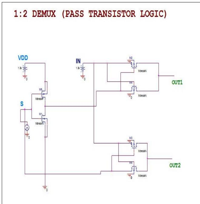
Fig. 3. Schematic diagram of pass transistor logic configuration of 1:2 de-multiplexers.
