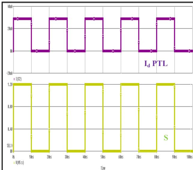
Fig. 6. Output current level for pass transistor architecture of 1:2 demultiplexer 1.2V VDD
