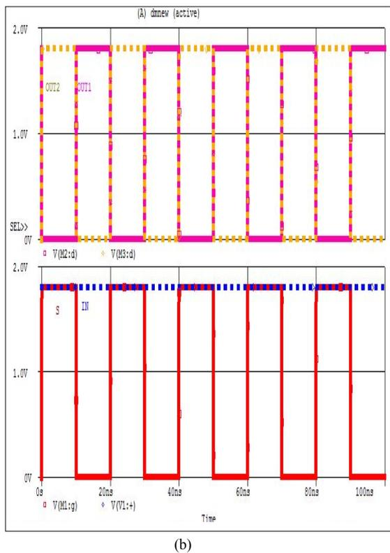
Fig.1. Simulated gate level structure and Characteristic for 1:2 demultiplexer (a) gate level structure and (b) Input and output voltage results.
