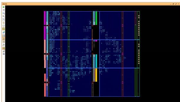
Fig. 5 device level diagram of 32 bit multiplier with Kogge Stone Adder
