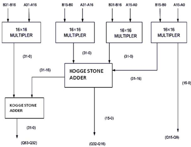
Fig 4:  $32 \times 32$  Vedic Multiplier with Kogge Stone Adder
