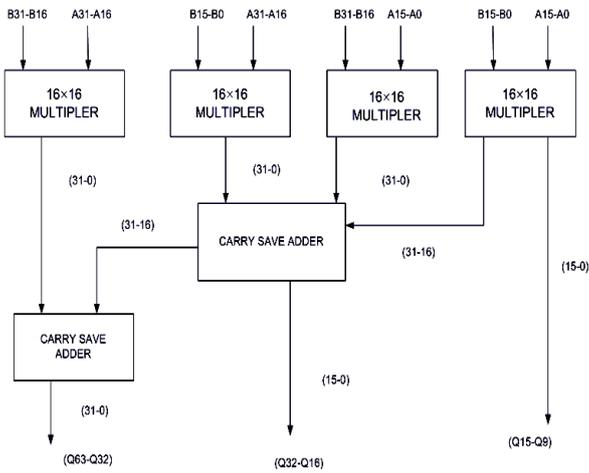
Fig 3:  $32 \times 32$  Vedic Multiplier with Carry save Adder
