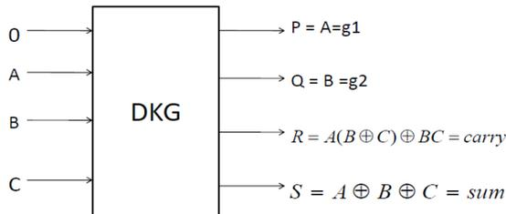
Fig. 6b DKG gate as a Full adder
