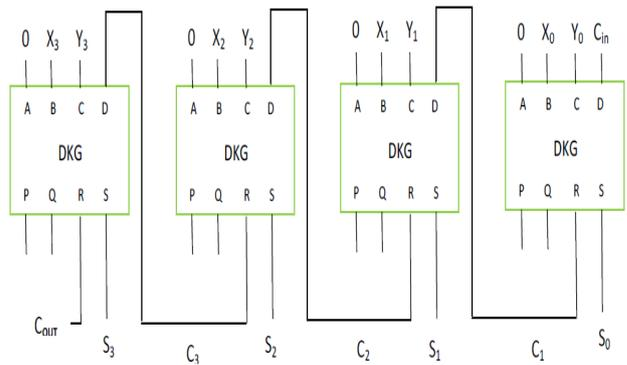
Fig. 6c Parallel adder using DKG gate
