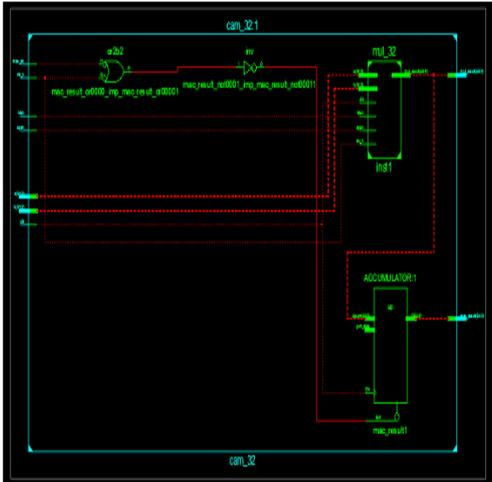
Fig 7: RTL schematic of 32 bit MAC architecture
