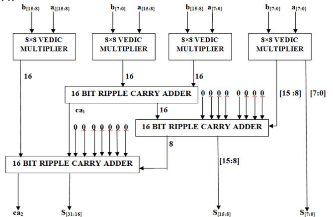
Fig 2: 16×16 Vedic multiplier using 8×8 Vedic multiplier
