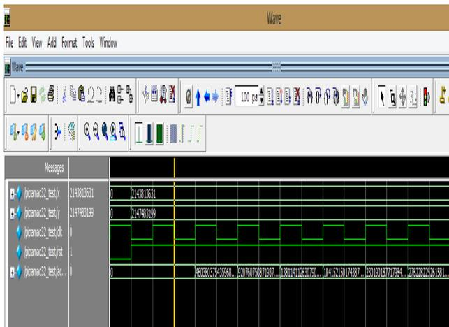
Fig 9: 32 BIT MAC simulated output in modelsim 6.5b
