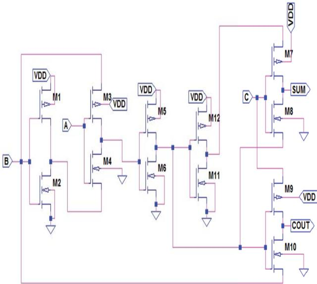
Fig.5(b). Schematic Diagram of Adder Cell Using GDI Logic Style
