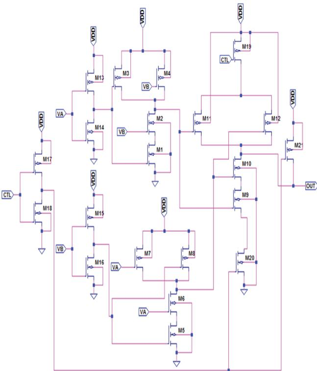
Fig.6(a) Schematic Diagram of MXOR Cell Using CMOS Logic Style
