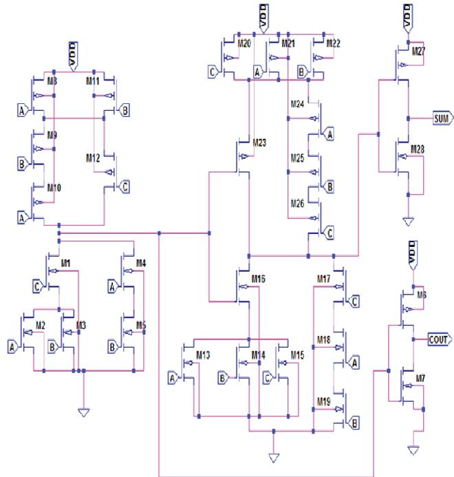
Fig.5(a). Schematic Diagram of Adder Cell Using CMOS Logic Style
