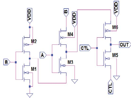
Fig.6(b) Schematic Diagram of MXOR Cell Using GDI Logic Style
