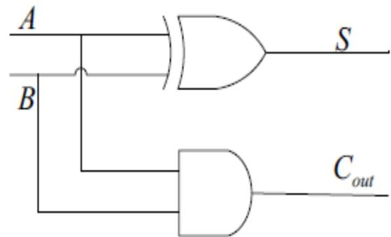
Figure 1.the logic circuit of half-adder
