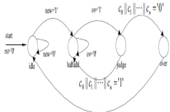
Figure 5. The state transition diagram for Barrel integer addition algorithm
