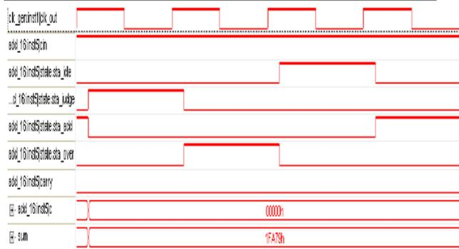
Figure 6 Timing Simulation of 16-bit adder
