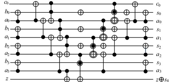
Fig. 3. Proposed reversible 4 bit adder with input carry
