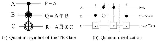
Fig. 2. TR gate and its improved quantum implementation
