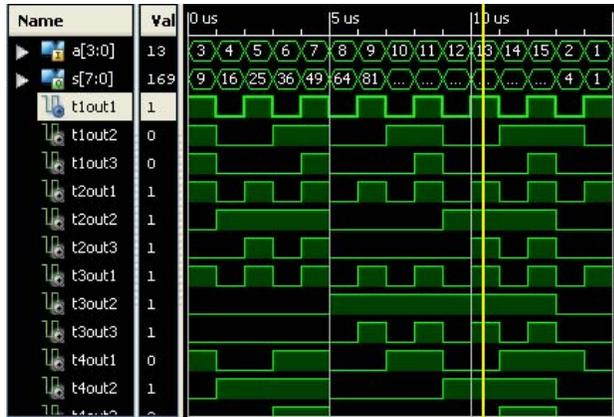
Fig. 13. Functional verification of 4x4 square unit
