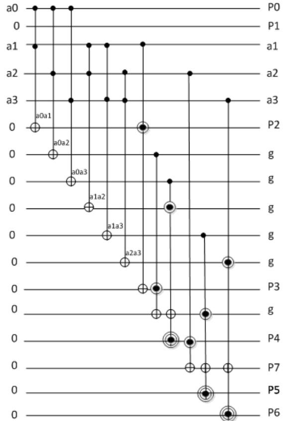
Fig. 11. Complete Reversible circuit of 4 bit square unit
