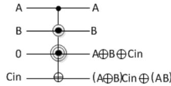
Fig. 9. DPG gate as full adder
