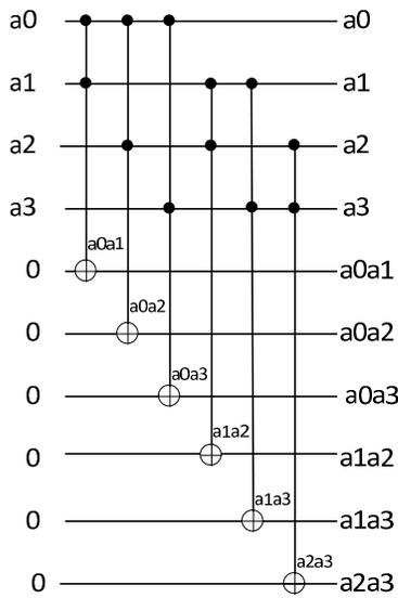
Fig. 7. Proposed reversible partial production generation circuitry for 4x4 square unit
