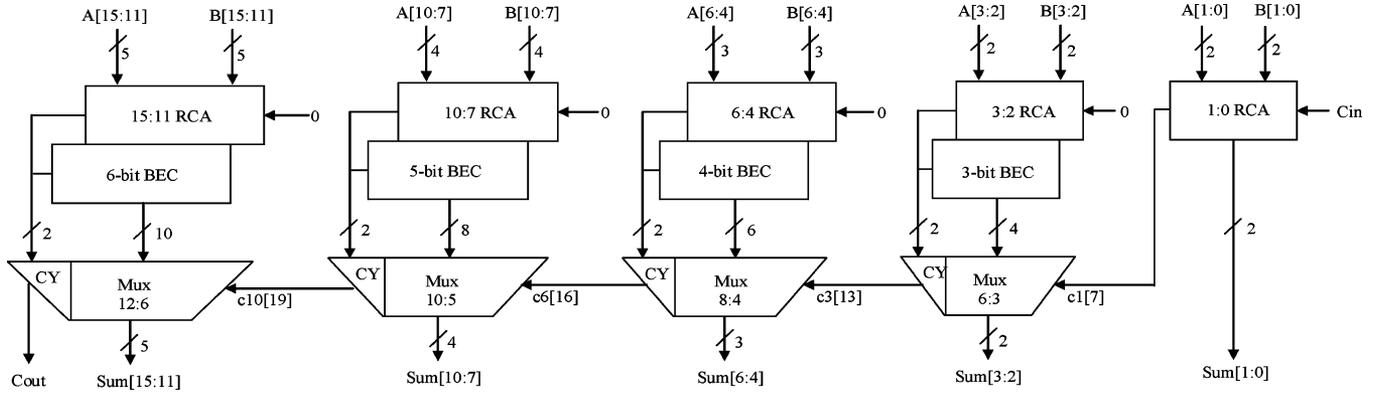
Fig. 6. Modified 16-b Sqrt CSLA. The parallel RCA with  $C_{in} = 1$  is replaced with BEC.
