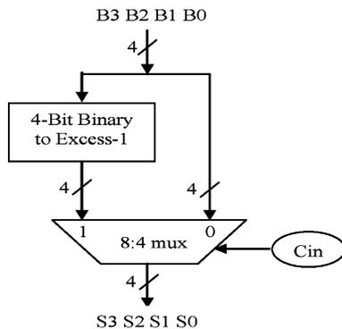
Fig. 3. 4-b BEC with 8:4 mux.
