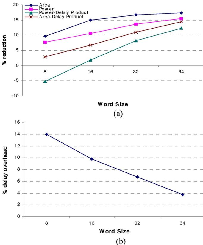
Fig. 8. (a) Percentage reduction in the cell area, total power, power-delay product, and area-delay product. (b) Percentage of delay overhead.
